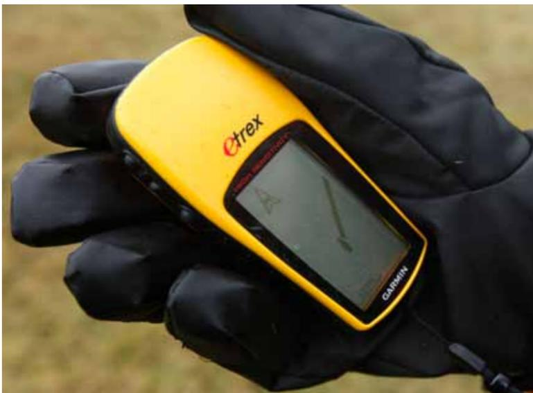
This feature records a track log while you are moving that, at any time, you can follow back along the same path. It is one of the most useful features, especially in poor visibility.
